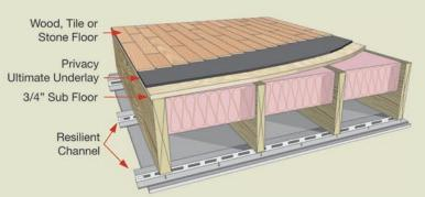
Privacy Ultimate Underlay adds significant mass to block airborne noise, while absorbing footfall noise; all in one step!
