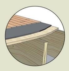
Under any floated engineered or laminate wood floor Privacy Ultimate Underlay is simply loose laid and taped; install floor immediately.
