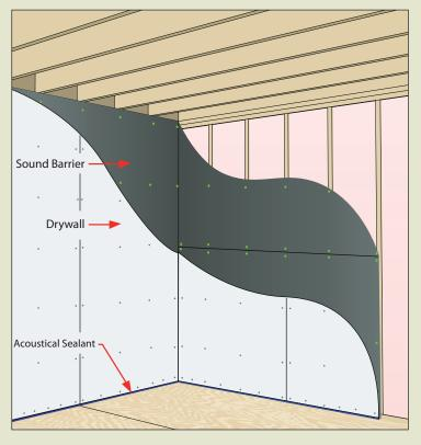
By attaching Soundproof Barrier directly to the studs, noise energy will be absorbed and redirected, lowering the noise level in the next room.
